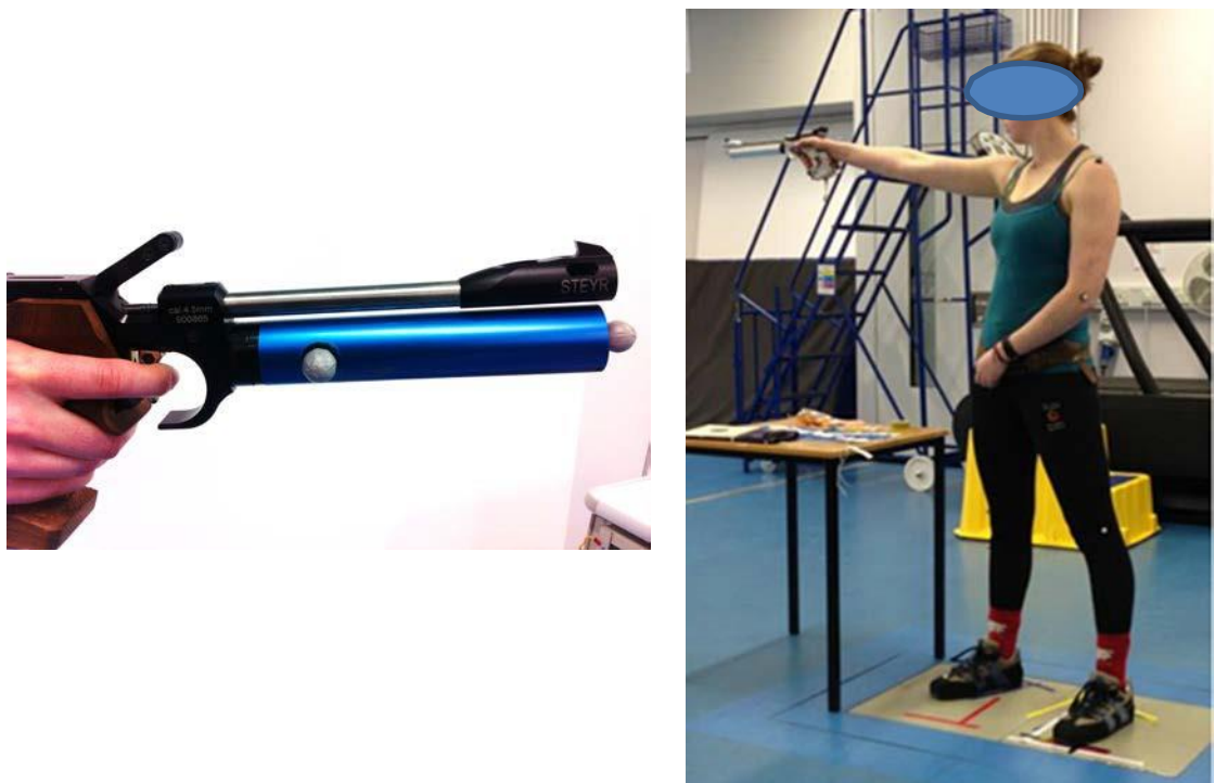
Figure 11.3. Placement of the additional markers on the pistol, and a participant shooting with the body and pistol marker set.
