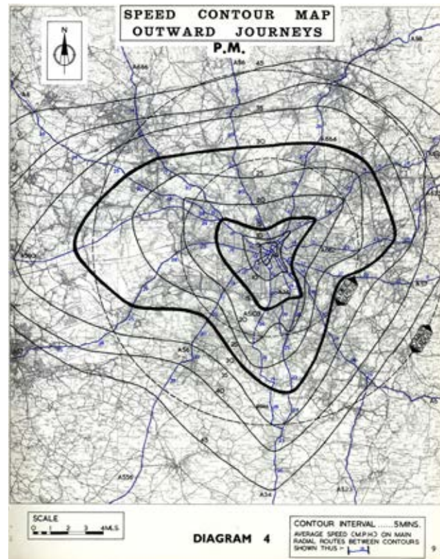
ABOVE. Fig.2.011. Illustrations of a desire map detailing the directions of major traffic flows and a contour plot of journey time. [Source: Author's scans from SELNEC [1962] A Highway Plan 1962 [Manchester: South-east Lancashire and North-east Cheshire Area Highway Engineering Committee], p.8, 21]
