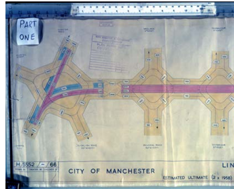
ABOVE. Fig.2.009. Diagrammatic representation of Link Road 17/7 showing origin – destination traffic volumes. This diagram is from 1958 and emblematic of the depth of statistical analysis and pre-planning that went into justifying the scheme. [Source: City Surveyor and Engineers plan archive, ref. 5552/-/xx?, GMCRO. Author’s scan, courtesy of Manchester Archives and GMCRO]
