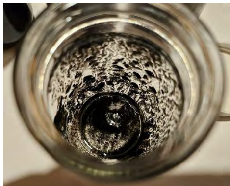
Figure 30 Image of the base of an emptied 0.001% concentration (w/w) SWCNT solution with dispersant showing giant clumps of CNTs at the base of the jar
