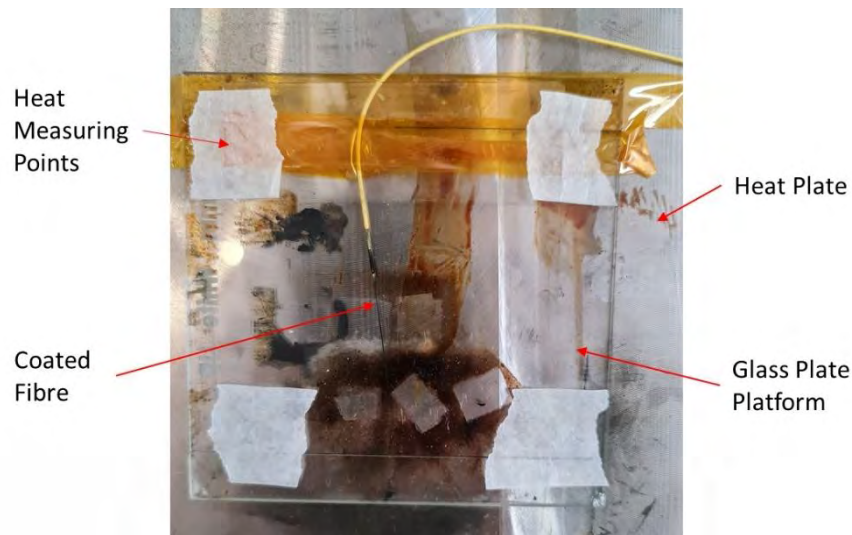
Figure 22 Example Coating Setup for the prepared SMF-28 Fibre with masking tape on the four corners of the glass plate platform for temperature measurements
