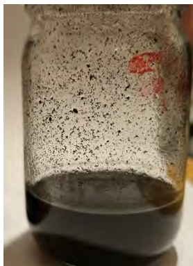
Figure 31 Image of a 0.0005% concentration (w/w) SWCNT solution with dispersant showing minor adherence to the inside of the jar
