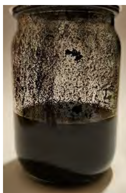
Figure 29 Image of a 0.005% concentration (w/w) SWCNT solution with dispersant that is half-poured showing large clumps of SWCNT adherence to the inside of the jar
