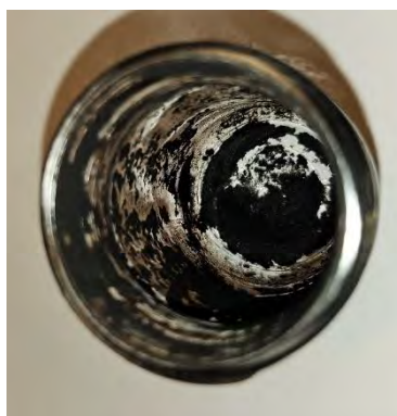
Figure 26 Image of an emptied jar of 0.005% concentration (w/w) SWCNT solution showing severe adherence of SWCNTs on the inside with huge clumps of SWCNTs at the base.
