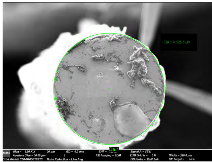
Figure 51 SEM imagery of the 3cm double coated SWCNT-SMF cross-section showing an approximate 0.5µm thick SWCNT coating around the 125 ± 0.7µm cladding diameter of the SMF-28
