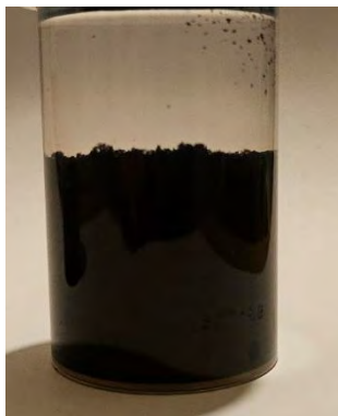
Figure 28 Image of a jar of 0.00025% concentration (w/w) CNT solution showing minor adherence of CNTs to the inside surface of the jar and splitting of the CNT and IPA-Water.
