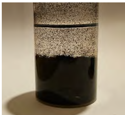
Figure 27 Image of a jar of 0.0005% concentration (w/w) SWCNT solution showing some adherence of SWCNTs to the inside surface of the jar with splitting between the SWCNT and IPA-Water.
