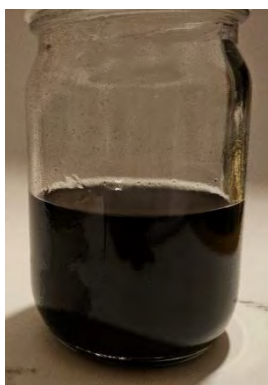
Figure 32 Image of a 0.00025% concentration (w/w) SWCNT solution with dispersant with minimal SWCNTs adhered to the inside of the jar.
