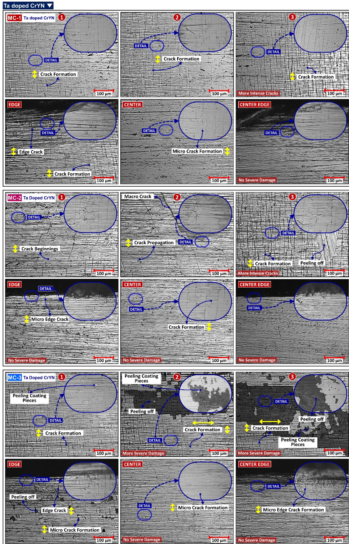
Fig. 15. 4-point bending optical microscope images of Ta-doped CrYN coatings (MC-1, MC-2 and MC-3)
