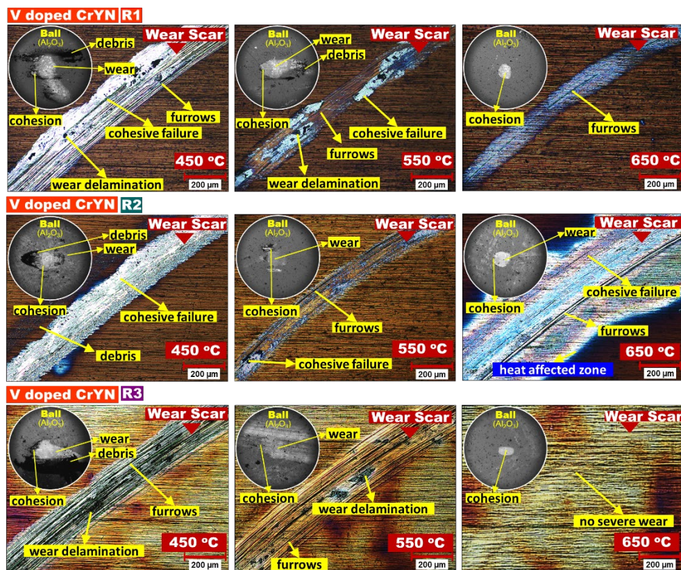
Fig. 19. Wear scars on V-doped CrYN coatings and the corresponding wear tracks on \text{Al}_2\text{O}_3 pins after annealing at 450 °C, 550 °C, and 650 °C.
