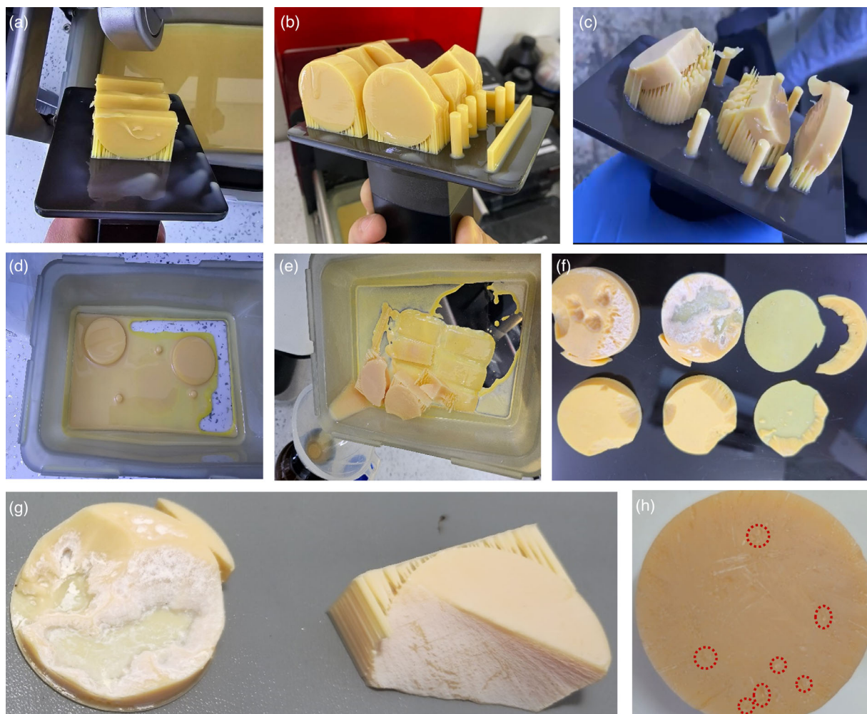
FIGURE 9 Different types of printing errors due to sample size: (a, b, c), Failure in printing the final layers of large samples with a high percentage of filler due to the excessive height of the samples, which is too long to print, leading to increased filler precipitation in the final layers. (d, e, f) Falling samples due to high suction and low adhesion between the samples and the plate. (g) Precipitations of the nanotube leading to printing failure due to high suction, (h) void entrapment within printed layers.
