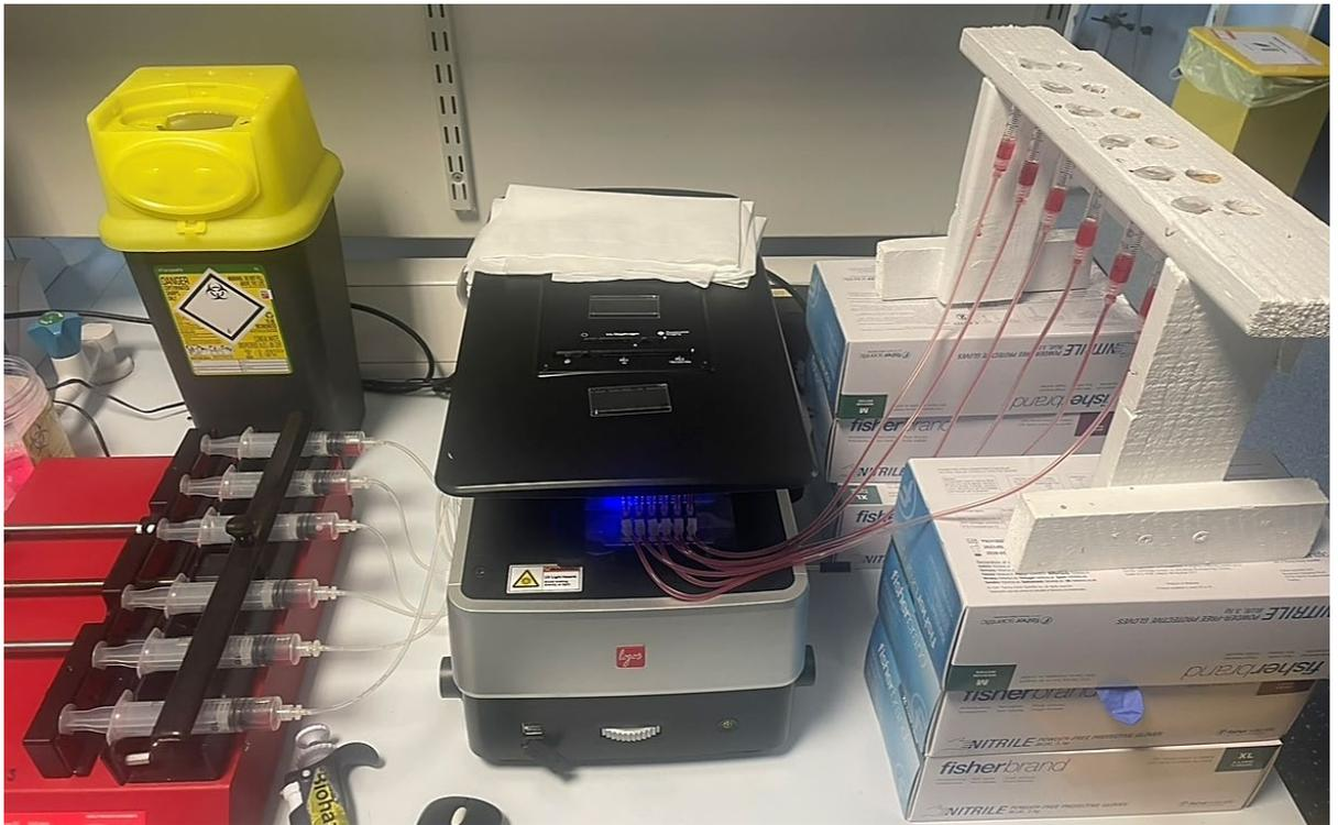
**Figure 2.10.** Picture of the endothelialised arterial thrombus formation model setting.
