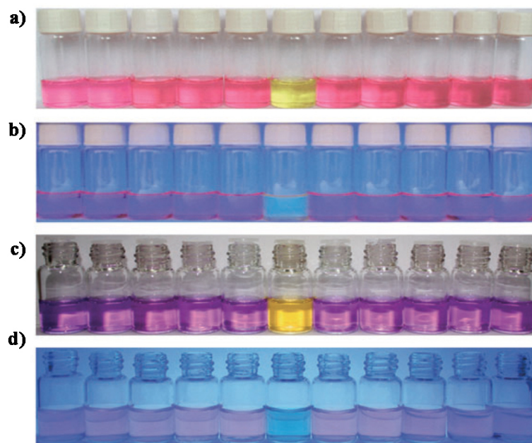
Figure 12: The naked-eye color changes of 35 (a and b) and 36 (c and d) in the presence of different anions (6 th cuvette for \text{HSO}_4^- ) under daylight and sunlight respectively. (Reprinted with permission from Ref 137. Copyright 2013, Royal Society of Chemistry).
