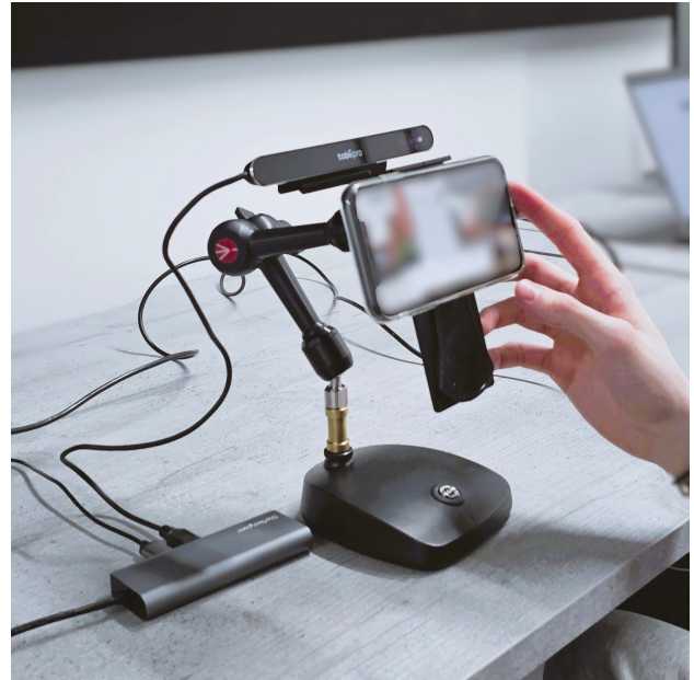
Figure 1: Tobii Pro Nano Eye Tracking Set Up with Tobii Pro Mobile Testing Accessory).
