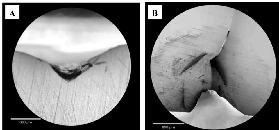
**Fig. 7.** Optical microscope images of edge chipping at 0.5 mm. (A) LU, (B) CT. Magnification  $4\times$ , scale bar = 890  $\mu\text{m}$ .
