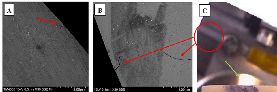
**Fig. 5.** Shallow indentation and cracks visible only under SEM  $\times 30$  (red arrows) (A) VCP (0.5 mm) (B) CT (1 mm) (C) Indentation with visible crack and bulging of the edge from plastic deformation (green arrow).
