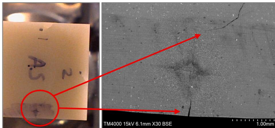
**Fig. 6.** Images of CT (1 mm) showing indentation with visible cracks (SEM  $\times 30$ ).
