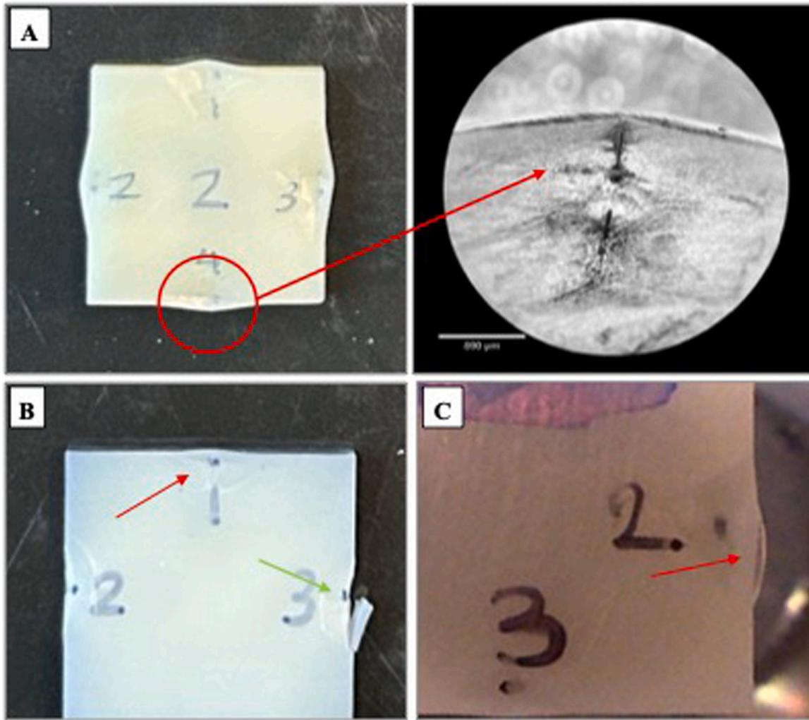
**Fig. 2.** (A) TC specimen after edge testing at 0.5 mm. Deep indentation and bulging of the edge are clearly noted. (B) A close up of one of the edges under optical microscope ( $\times 4$ ) showing no cracks. (C) DT specimen after edge testing at 0.5 mm. Red arrow shows indentation and deformation of the edge. Green arrow shows incomplete chipping. (D) ND specimen after edge testing at 0.5 mm. Deep indentation and bulging is observed.
