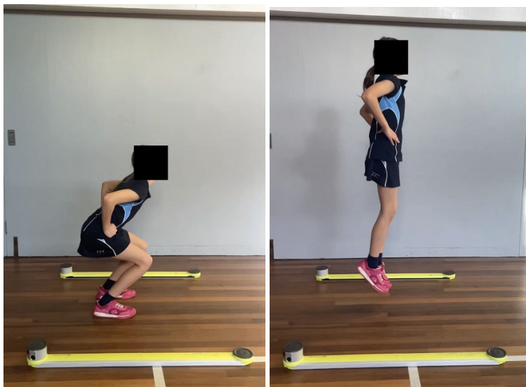
Fig 3.1 Illustration of the participant's starting position and location of the Optojump Next system during a squat jump (SJ).
