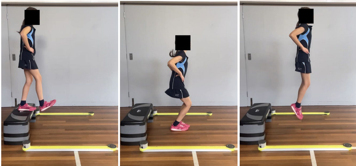
Fig 3.3 Illustration of the participant's starting position and location of the Optojump Next system during a drop jump (DJ) from a 30-cm step.
