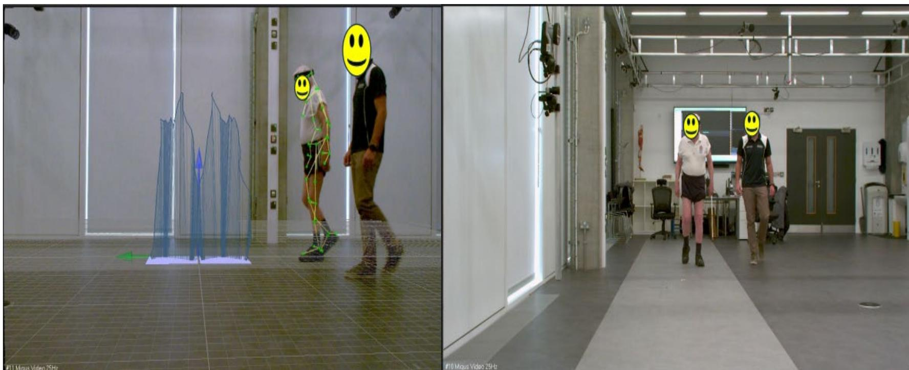
Figure 1 - Sagittal (left) and frontal (right) views of a patient with model and force vector overlay
