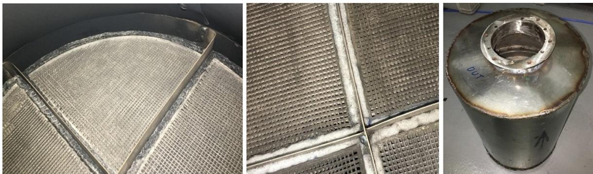
Figure 24: A commercial size 3D printed catalytic converter, tested under industrial conditions, taken from a publication by A. Doyle et al.<sup>156</sup>
