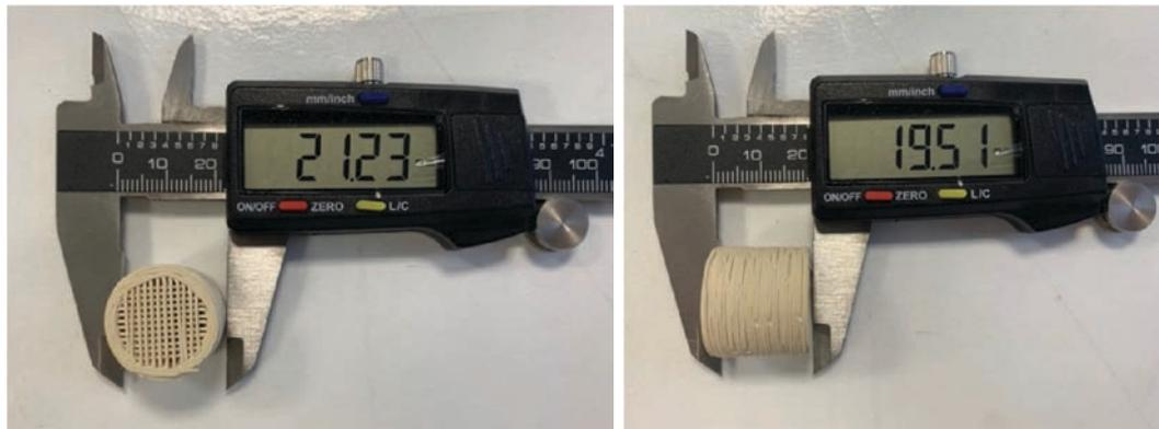
*Figure 66: Images of the printed robocast substrates being measured using a microcaliper .*
