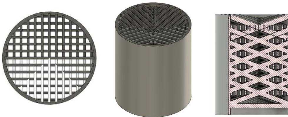
Figure 62: CAD design of a 0.5 mm, 15° fibre rotation in the Z-plane monolith.
