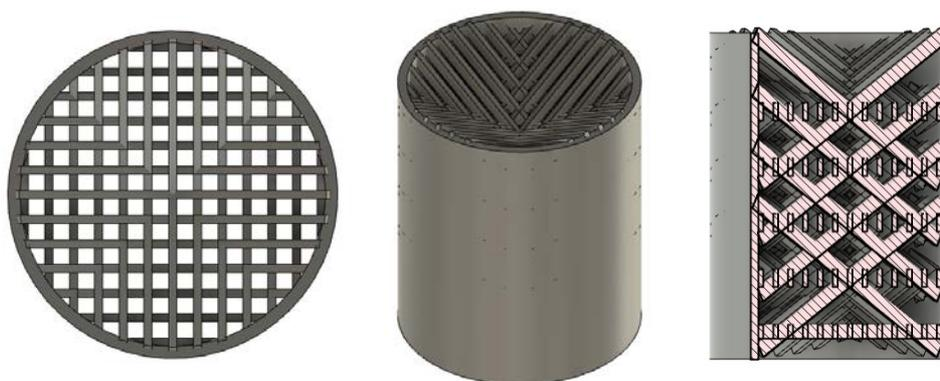
Figure 63: CAD design of a 0.5 mm, 30° fibre rotation in the Z-plane monolith.
