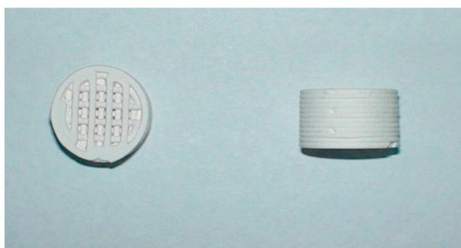
*Figure 22: An image of the 3D printed cylindrical monolith taken from the publication by C. Leclerc and R. Gudgila referred to above.<sup>155</sup>*
