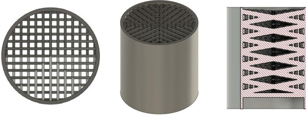
Figure 60: CAD design of a 0.5 mm, 7.5° fibre rotation in the Z-plane monolith.
