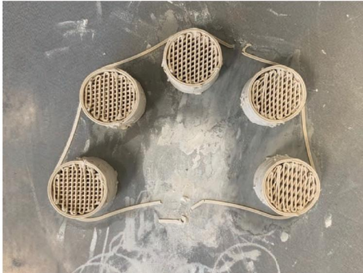
Figure 39: Image of the robocast substrates printed, with a variation in the X-angle, before post-processing.
