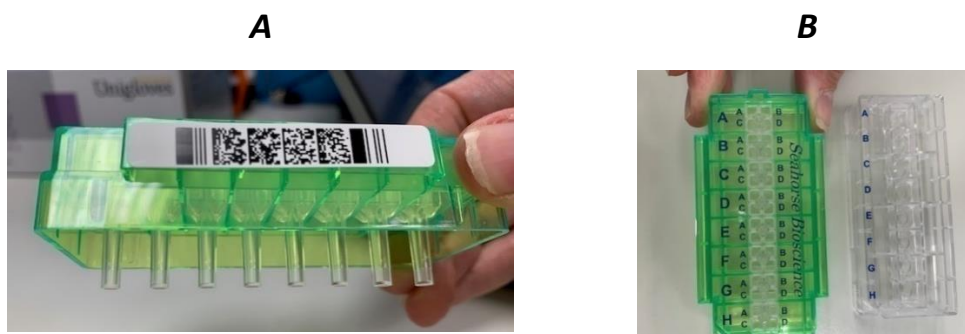
Figure 2-15: Seahorse sensor cartridges. A: sensor cartridge being lifted from utility plate. B: Utility plate next to sensor cartridge
