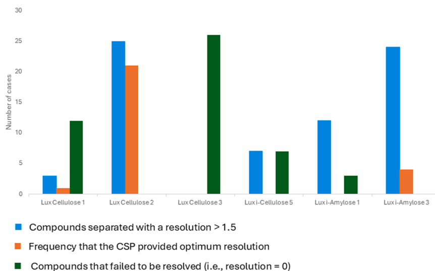
Fig. 3. Chiral performance of the CSP against the 26 chiral monosubstituted diphenidine racemates (1–10). ■ Compounds separated with a resolution > 1.5. ■ Frequency that the CSP provided optimum resolution. ■ Compounds that failed to be resolved (i.e., resolution = 0).
