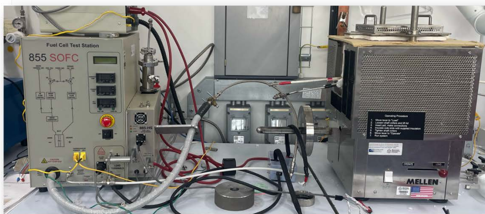
Figure 5.2: SOFC test rig, featuring the 855 SOFC test station with potentiostat 885 (left) and furnace (right).
