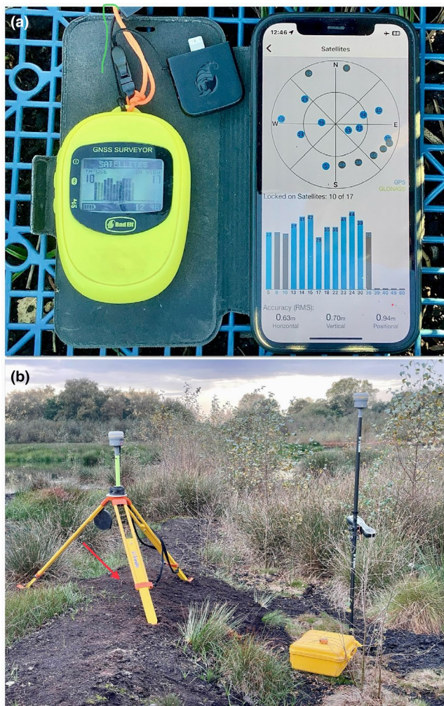
FIGURE 1 (a) Mobile GNSS receivers, iPhone, Bad Elf for Lightning Connector (BELC) (black) and Bad Elf Surveyor (BES) (yellow). The app shows data transmitted from the BES via Bluetooth—the available satellite constellation (grey) and the strongest satellite signals (light blue) used for trilateration and estimated horizontal accuracy. (b) Tripod mounted Trimble R10 located vertically above the base station ground peg (red arrow), the R10 Rover and the narrow east-west running bund—the south-north running bund is visible left off the ground peg.
