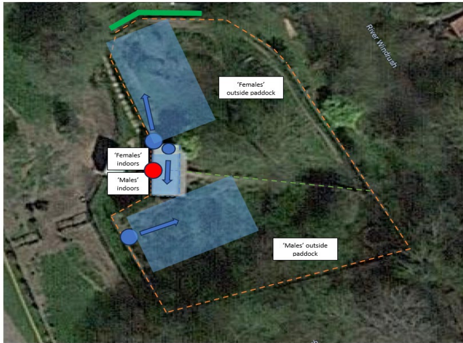
Figure A2: Networked CCTV coverage of the southern cassowary enclosure – Birdland. Blue circles indicate the locations of the cameras and the arrows the direction in which they are pointing. The light blue areas indicate the range that can be seen on each camera. Red circle indicate the locations of the sound recorders. Green line shows the public viewing areas. Orange dashed line shows the enclosure boundaries.
