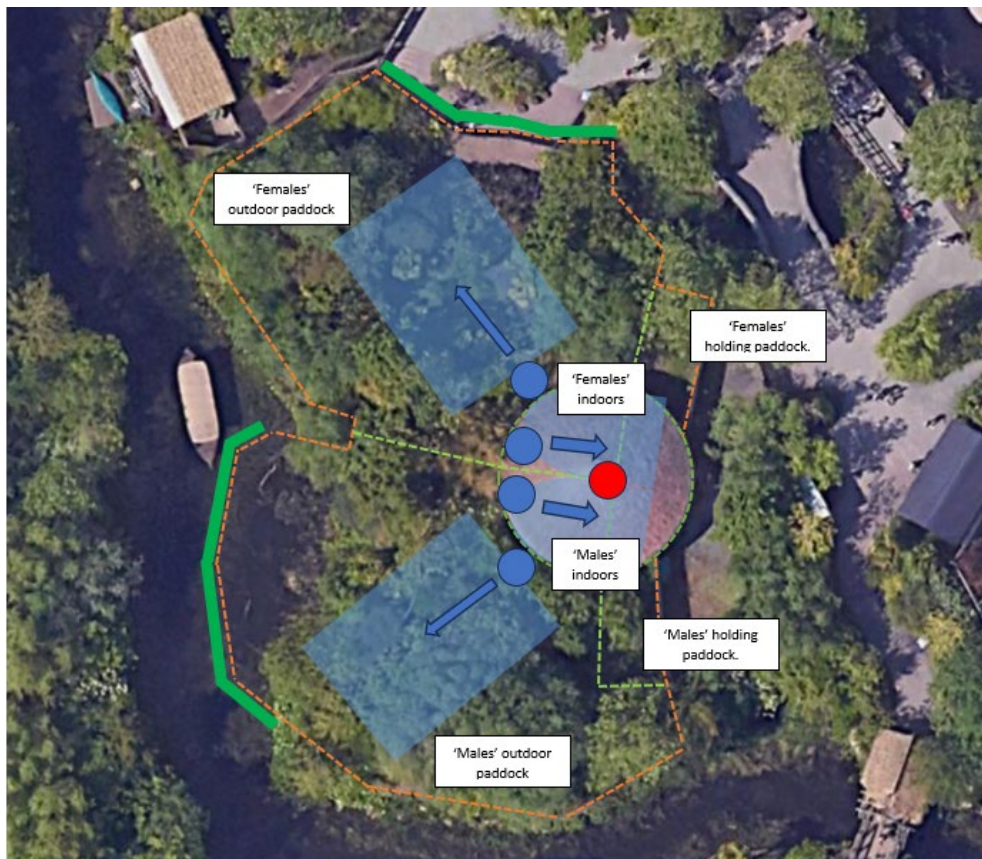
Figure A2: Networked CCTV coverage of the southern cassowary enclosure – Birdland. Blue circles indicate the locations of the cameras and the arrows the direction in which they are pointing. The light blue areas indicate the range that can be seen on each camera. Red circle indicate the locations of the sound recorders. Green line shows the public viewing areas. Orange dashed line shows the enclosure boundaries.
