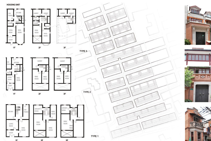
Fig. 2. Sample image showing part of the survey conducted in Siming Village, showcasing a roof plan of the street, existing typologies and gates and facades details.
