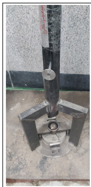
Figure 5. RDWI test device.
