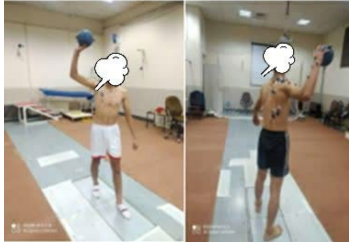
Fig. 2. Recording ground reaction force data during throwing
