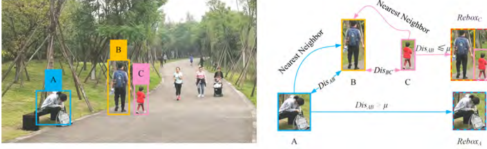
Figure 4: Example diagram of nearest neighbor interaction. Take A and B for example, we find their nearest neighbor C according to their distances among individuals. Then, we crop individuals and their nearest neighbors based on the threshold \mu . Finally, we extract features of the Rebox regions as every individual's feature.
