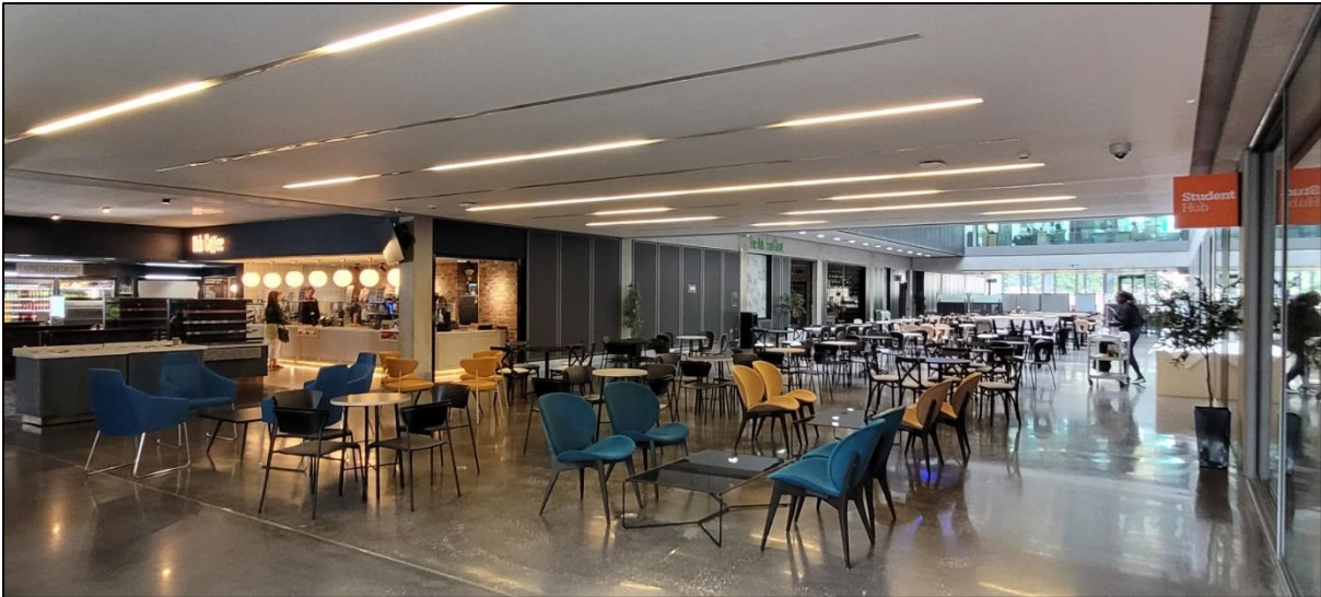
Figure 3.17. The open plan of the atrium and canteen, illustrating how thermal losses can be large due to nothing stopping the air flow.
