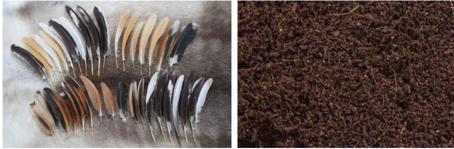
FIGURE 1: Fresh Gallus-Gallus fibres and waste coir powders.
