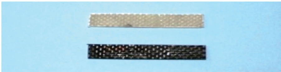
FIGURE 4: Dynamic mechanical analysis specimen of specially treated selective Gallus-Gallus fibres reinforced polyester polymer composite and neat polymer composite.
