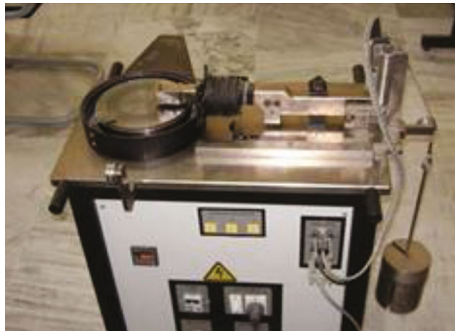
FIGURE 3: Wear testing arrangements in the pin-on-disc apparatus.
