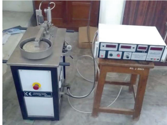
FIGURE 7: Pin-on-disc tribometer setup.
