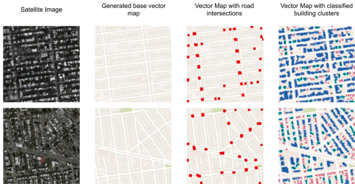
Fig. 14. Some samples of generated vector map with marked road intersection and classified building clusters.
