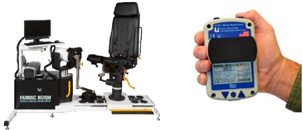
Fig 1. Isokinetic dynamometer (left) and Lafayette handheld dynamometer (right). Photos used with permission from copyright owner.
