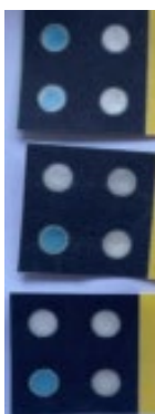
Figure 5.3. Image of replicates obtained for sample 1 (MDMA and 4-CMC) depicting the identification of MDMA on all three replicates and one false negative result for 4-CMC
