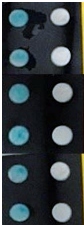
Figure 5.2 Image of replicates obtained for sample 18 (amphetamine) depicting the identification of amphetamine. The top left well on the black tab contains the anti-methcathinone antibody, as there is no 4-MMC present within sample 18 then the response from TMB is the most intense colour (blue) that can be observed by eye. The top right well on the black tab contains the anti-amphetamine antibody: as amphetamine is present within sample 18, the TMB subsequently produces a lower response as the unlabeled target antigen (amphetamine) out competes the labelled amphetamine-HRP for the active sites of the anti-amphetamine antibody
