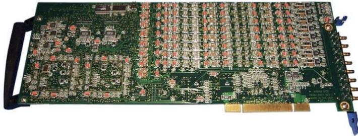
*Figure 4-7. PCI-8, 8-Channel acoustic emission system on a board*
