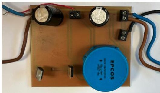
*Figure 4-1. IGBT-based DC-DC boost converter.*
