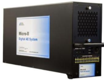
*Figure 4-8. Micro II Acoustic Emission data acquisition computer*
