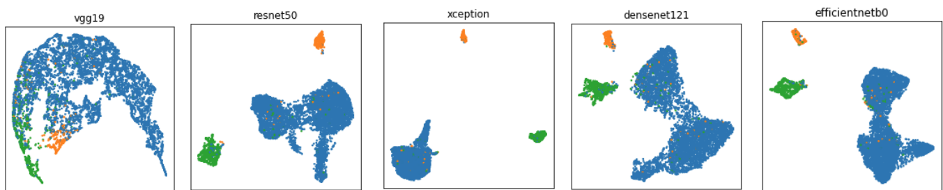
Figure 5. Visualization of full dataset feature distributions extracted with VGG19, ResNet50, Xception, DenseNet121, and EfficientNetB0. These graphs visually illustrate the separability of three anatomic sites.
