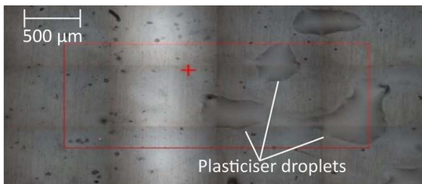
Figure 5.11: Optical microscopy image of exudation on a plasticised PVC sample.
