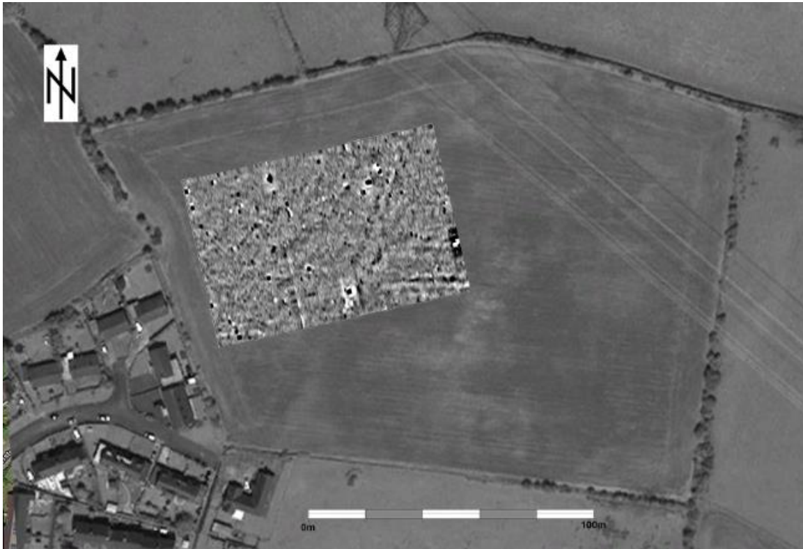
Figure 107: Geophysical survey results superimposed on satellite image of the site, Penbodeistedd (Llanfechell).
