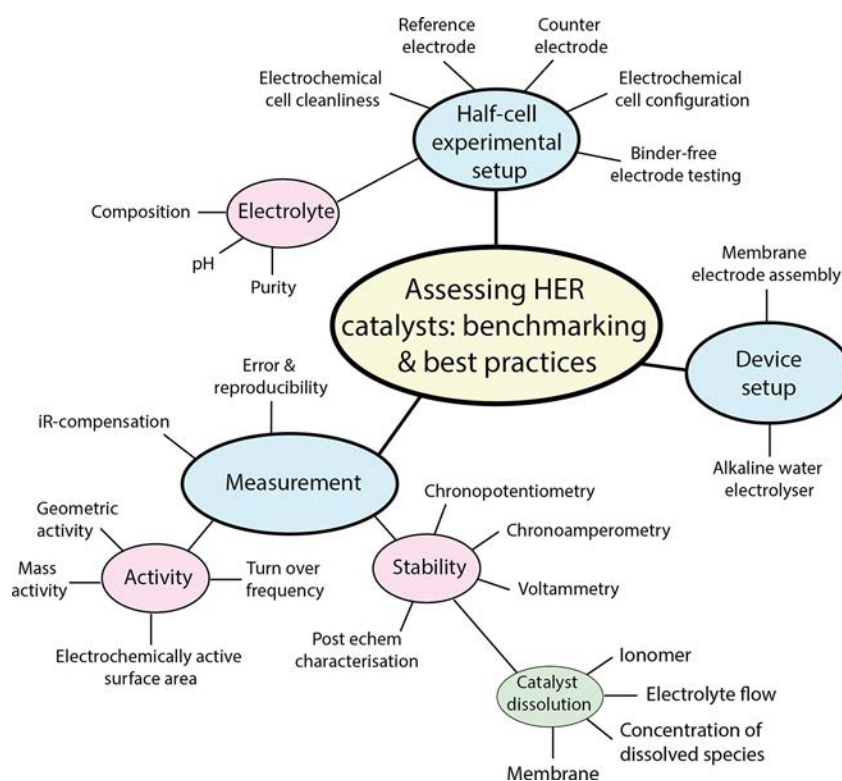
Figure 4. Schematic to highlight the key considerations that a researcher should factor into the design of their HER catalyst performance measurements.
