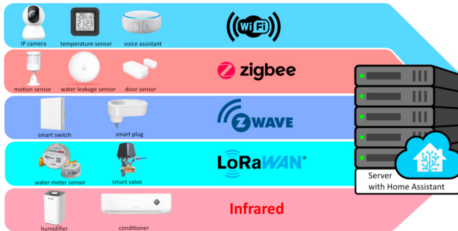
Fig. 1. Architecture of multi-layer integration of wireless protocols.
