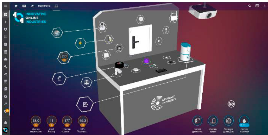
Fig. 3. Digital twin of the “Smart Home” testbed and Home Assistant platform control panel
