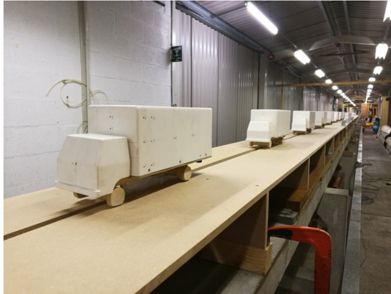
Figure 3 The lorry platoon model and the suspended ground plane used in the moving-model experiments
