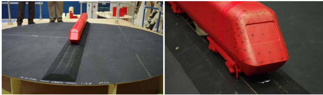
(a) The wind tunnel model and setup
