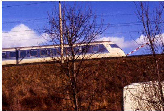
(c) The TRANSAERO full-scale Inter-Reggio measurements (author photograph) showing wind measurement boom at front of train
