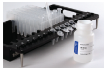
Setup and configuration of deck trays. Nuclease-Free Water is added to the elution tubes as shown. Plungers are in well #8 of the cartridge.
