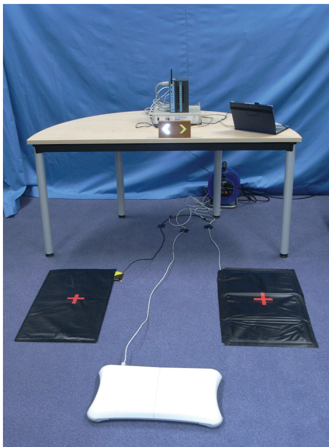
Figure 2. Set up of the LBRTT test (Spiteri et al., 2013).
