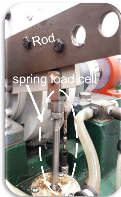
Figure 24 - Hydraulic dynamo-meter rod, and spring load cell.
