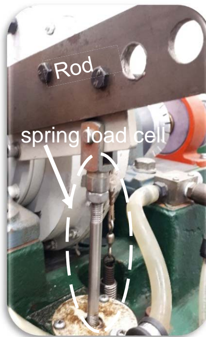
Figure 24 - Hydraulic dynamo-meter rod, and spring load cell.
