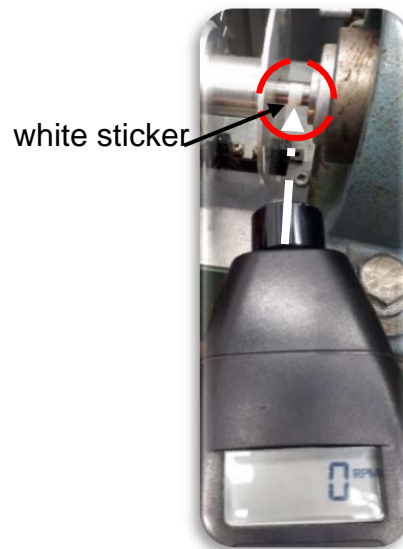
Figure 26 - The tachometer is positioned close to the rotary disk to detect the white sticker, which indicates the instantaneous rpm speed of the engine.
