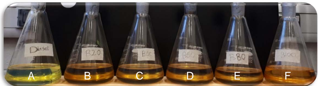
Figure 28 - 200 ml of A) Diesel, B) WCO B20, C) WCO B40, D) WCO B60, E) WCO B80, and F) WCO B100
