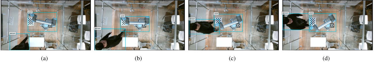
Fig. 9. Images with annotation information in the real dataset. From (a) to (d), the whole process of human–robot collaboration is captured from the Kinect V2 sensor mounted on the top of the UR10.
