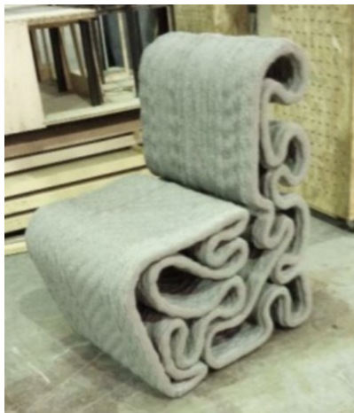
Figure 2 A hollow form 3D printed chair using mortar
