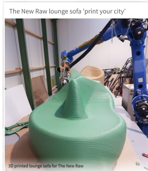
Figure 13 3D printing technology using a large robotic arm to print a sofa (10-xl, 2022)
