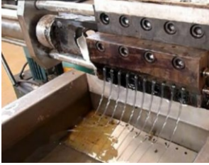
Figure 9 The extruder head, extruding 10 filaments that will be cut into pellets.
