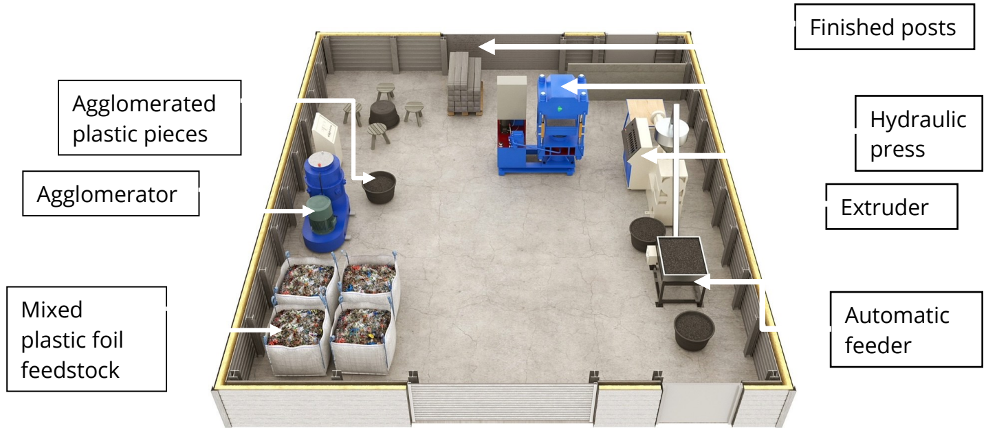
Figure 3 Layout of IEM basic single line plant with 150 tonne per year capacity
