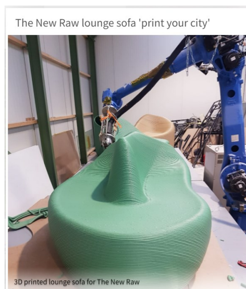
Figure 17 3D printing technology using a large robotic arm to print a sofa (10-xl, 2022)
