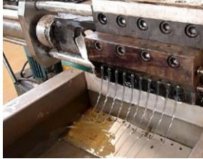
Figure 13 The extruder head, extruding 10 filaments that will be cut into pellets.
