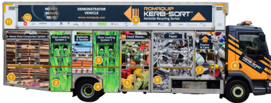
Figure 11 A specialist Romaquip kerb-sort waste truck for second stage kerbside pre-sorting ( https://www.romaquip.com/kerb-sort )
