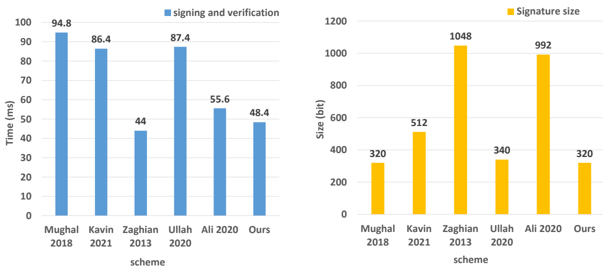
Figure 3. Comparison of computational and communication costs of our proposal with Mughal 2018 [23], Kavin 2021 [31], Zaghian 2013 [26], Ullah 2020 [41], and Ali 2020 [42] schemes.
