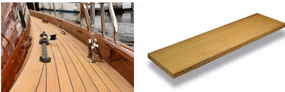
Figure 1.3 Appearance of Lignia® Boat-Deck (22-year-old resin impregnated Monterey pine boards) (Reproduced from [5])
