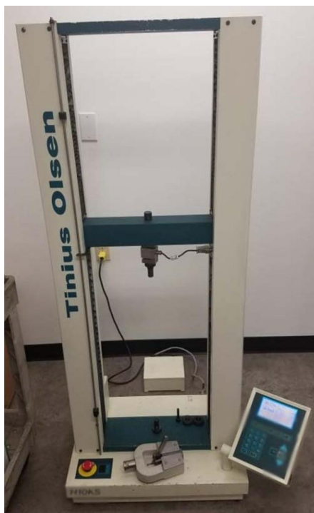
Figure 2.6 Tinius Olsen H10KS tensiometer.
