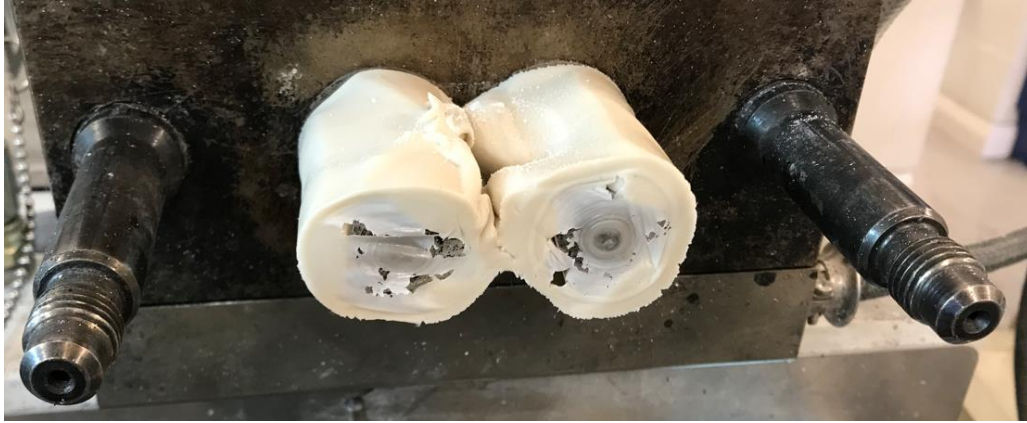
Figure 2.2 PVC formulation containing hollow calcium carbonate filler (19 wt.%) after rheometric mixing
