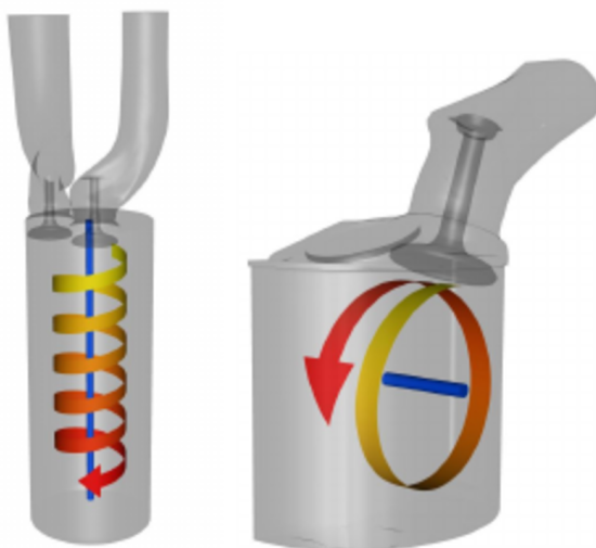
Figure 1.2: The swirling motion of flow in the combustion chamber of a diesel engine Swirl
