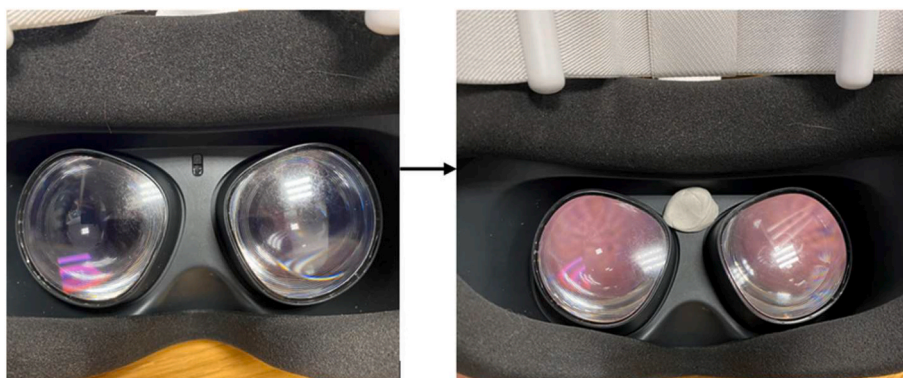
Fig. 3. Covering the proximity sensor which is located between the two eye lenses.
